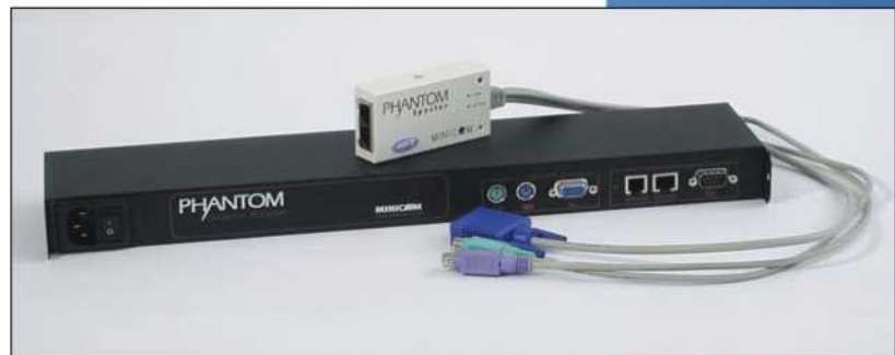
Universal Phantom Manager with Specter Unit
